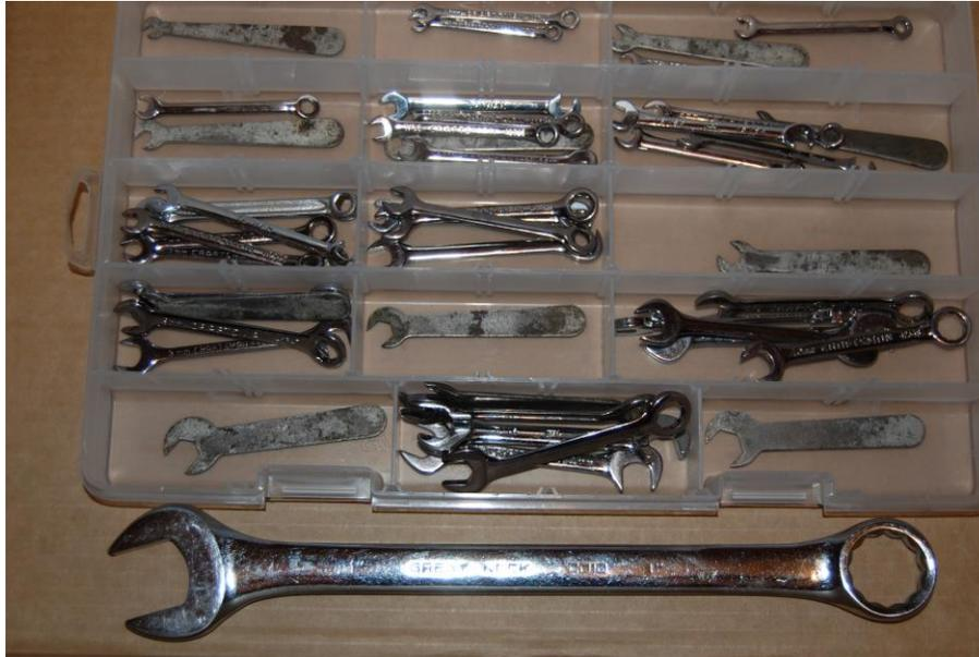
Unless you work on large machines, you probably won't need a 1" wrench as shown at the bottom. Ignition wrenches were originally made for working on automotive ignition systems, but are useful when tightening small fasteners on a robot chassis or electronics panel.
