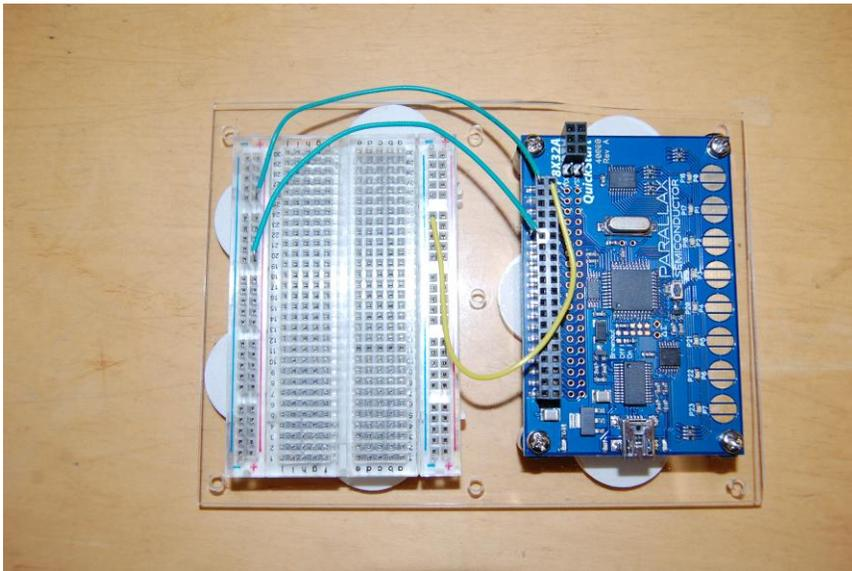
It can be used as a guide when cutting plexiglass with a special cutter to make board holders. Having both the microcontroller board and breadboard mounted together on a solid structure can make projects flow smoother, and have less problems with wires pulling out.
