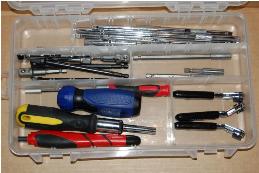
These are handles for the 5/32" and 1/4" drive screwdriver bits. A variety of different lengths is needed. Keep in mind, though, this type of screwdriver won't work in all situations, because they must have a sleeve for the bits to be inserted into. You may also need a regular set of screwdrivers (up to at least 8" long if possible), to have all situations covered.
