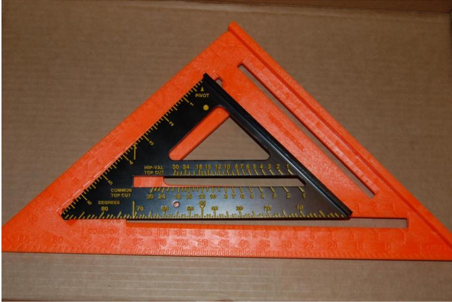
A speed square is useful when you are laying out project enclosures. Once the holes are laid out, you can use either a corded or cordless drill to drill them.
