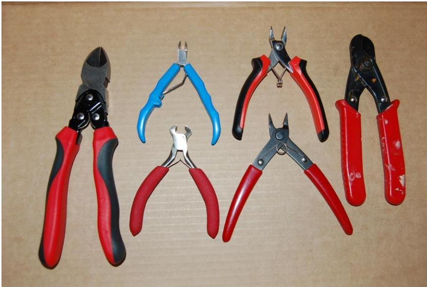
Wire cutters do just that. A variety of types are available. Diagonal cutters are needed. If you make circuit boards with through-hole components, a pair of flush cutters are needed to trim the leads sticking through. Cable cutters (right) make clean cuts through larger materials like coaxial cable.
