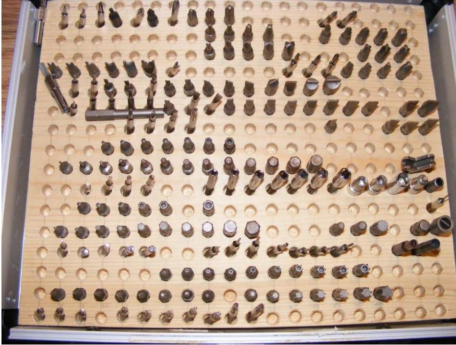
A variety of screwdrivers are needed. If you are making your own devices, you can usually choose the fastener you use. Usually a #2 Phillips and a flat screwdriver are needed. If you take apart existing equipment, you can run into about every shape of screwdriver you can imagine from Phillips to square to triangle, not to mention the "tamper-proof" drivers.
