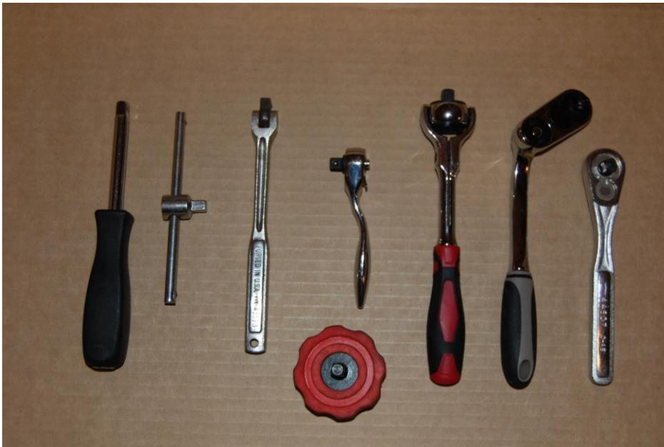
A variety of drive tools is useful, also. On the left is a spinner handle with a drive socket in the handle. It lets you turn sockets by hand, and the drive end lets you inset a sliding t-bar or breaker bar (next) to apply more torque. Tiny ratchets are needed for small places. Ratchets that let the head tilt or pivot are useful for hard-to-reach places.
