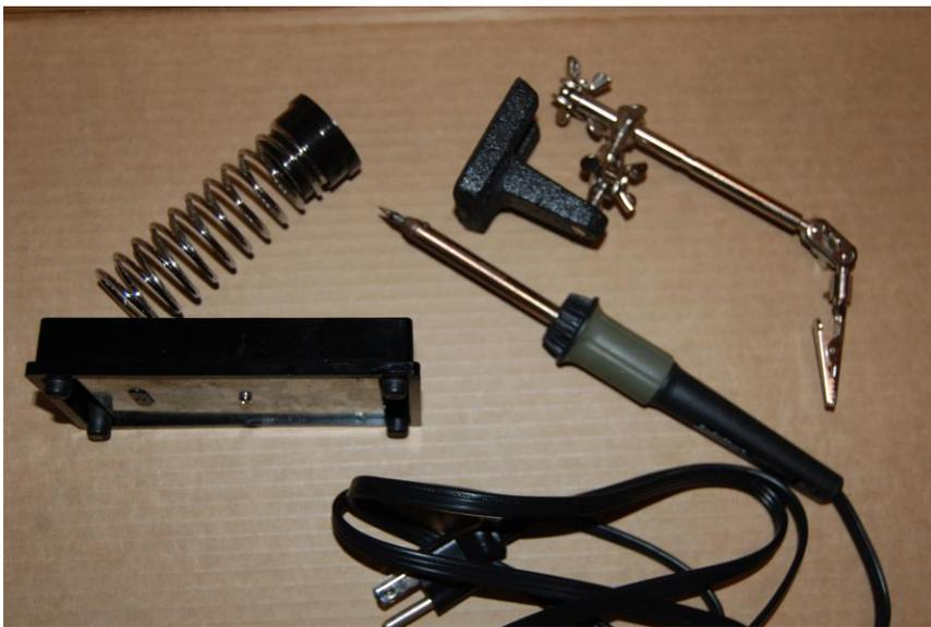
A soldering iron is needed for some assembly. A stand holds it out of the way. A "helping hands holder" can hold the circuit board or components while you solder them. Some of the cheap models are not made well and can move around in use.
