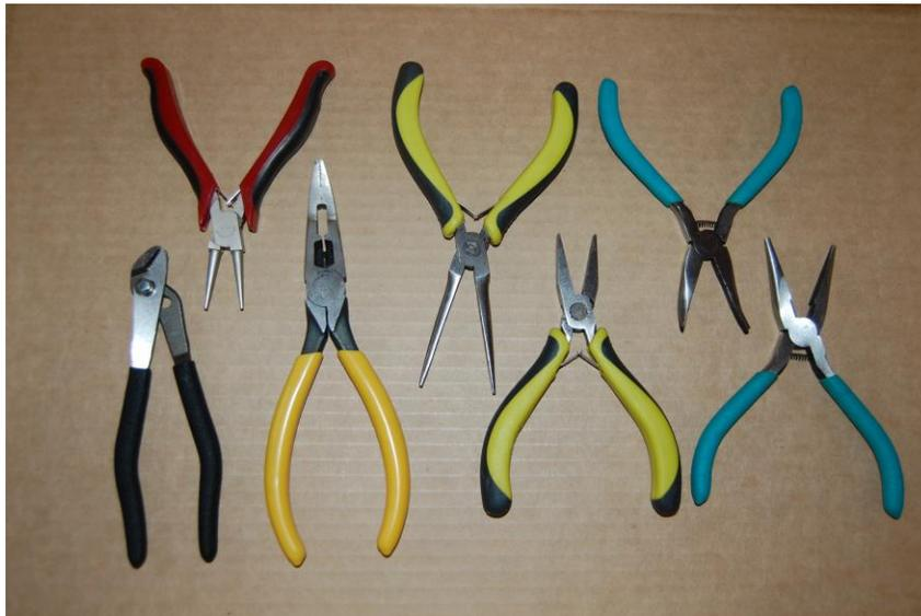
A variety of pliers are useful for holding materials. They can be used to hold a nut on a bolt while you get it started, but will probably slip off and cause damage if used for final tightening. Round jaw pliers can be used for forming resistor and capacitor leads.
