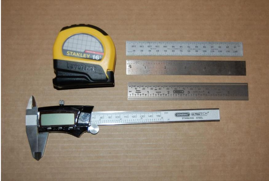
Rulers and tape measures are needed for measuring sizes and also for layout. Calipers are useful when trying to determine drill bit size for a component.
