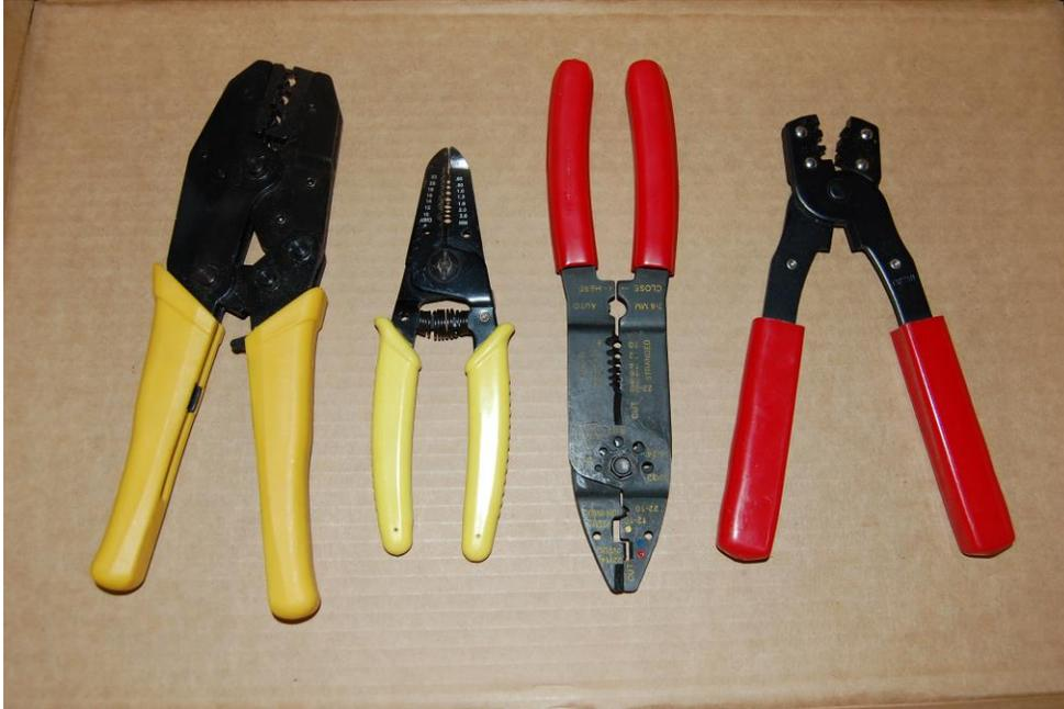
Wire stripping pliers (2) have notches for different sizes of wire, and let you remove the insulation without damaging the wire. Some crimping pliers are used for automotive type connectors (1,3), D-sub crimpers are used for D-sub connectors, telephone crimpers and Cat-5 crimpers are used for their connectors.
